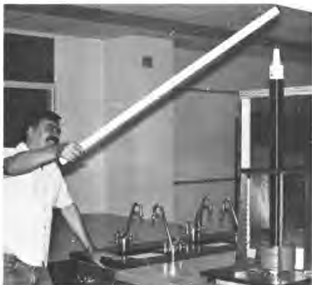
Fig. 5. Tesla coil demonstration. This version is too dangerous to take off campus. A smaller harmless Tesla coil (see reference) was constructed to take off campus.
