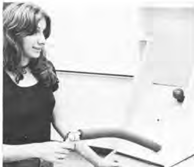
Fig. 6. The reaction timer. The 1/10-second clock is on back of the timer. The updated version presently under construction is all digital and will have all the electronics facing the student.
