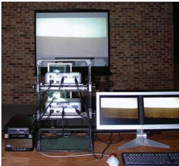
Fig. 2. The basic setup for a stereoscopic projection system includes a CPU with dual video output feeding two DLP projectors that project through orthogonally aligned Polaroid filters and are aligned onto a polarization preserving screen.
