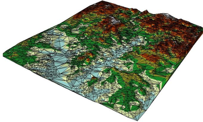
Figure 2. Triangular Irregular Network indicating the surface roughness-dissectivity.
