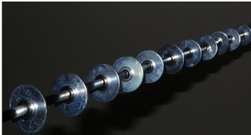
Fig. 2. Magnet-washer-magnet “particles” on the carbon fiber rod.
