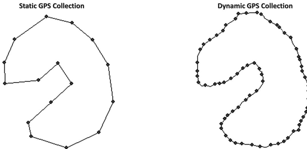
Figure 1. Static versus dynamic GPS data collection.
